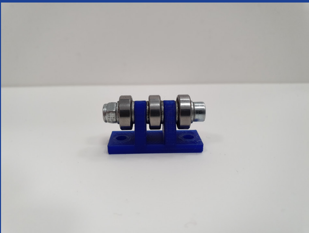
Caster made out of bearings
